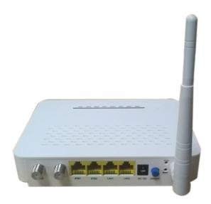
CD5204LW is the eoc slave based on HomePlug AV solution for Ethernet access over coax. It works together with eoc master which is based on HomePlug AV solution as well to construct a two-layer Ethernet data transmission channel on CATV coax cable, provide the Ethernet access service based on the existing coax cable networking.
